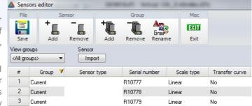
To make the sensor setup even more automated, our signal conditioning modules support TEDS, which is a standardized "smart sensor interface". TEDS is an acronym for Transducer Electronic DataSheet . It is a table of parameters (manufacturer ID, model number, serial number, version, and many more) that identifies the transducer.
