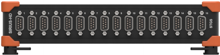
Illustration 145: HD-STGS with 16 DSUB-9 connectors
