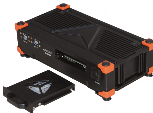
Illustration 56: SIRIUS-SBOX2 with removable SSD
