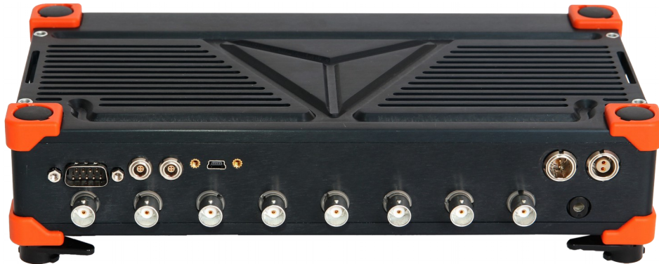
Illustration 55: Rear side connectors of the Analogue-out version
