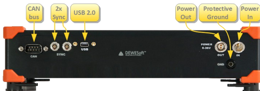
Illustration 20: SIRIUS chassis: connectors on the rear side
