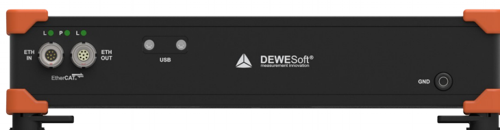
Illustration 52: Sirius EtherCAT® rear side connectors
