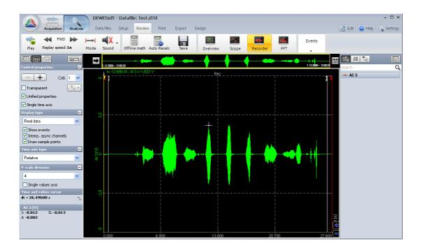
Now press the "**Offline math**" button ①. This will open the "Setup" tab sheet in Math section. Here you are able to add any math just like being in Acquisition (measure) mode.
