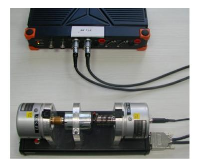
There are several encoder modes: The first one is used to measure only the *rising edges* of input A - this is the so called **X1** mode. The second mode - **X2** measures the *rising* and falling *edges* of input A while **X4** mode measures *rising* and
