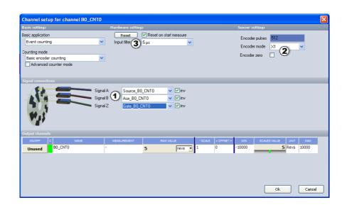
Now let's take some **measurements**. The *output* of this counter is the one that which counts *up* when signal A *leads* signal B, and counts *down* when signal B *leads* signal A. The *positive edges* of signal A is used *to calculate* the counts ④.
