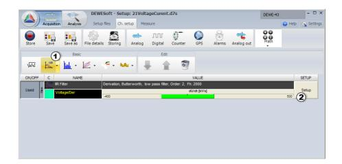
Now let's click the **Setup** button O to define the filter. We select Voltage O as the *input*, then selects the **d/dt** icon O for the calculation of the derivative. Then the user defines the units as **kV/s** and defines in Scale field the *scaling factor*. Normally, if the input unit is V, the output will be in V/s. Since the values will be simply too high, we set the unit to **kV/s** O and define the scaling factor as **0.001** O.
