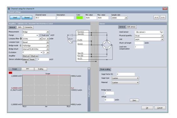
Next we set the Strain scaling to used and set the k factor of the gages to 2 and the Bridge factor to 2.6. The value of 2 is read from the strain gages *data sheet*. The value of 2.6 is a *bridge factor* from the table of bridge configurations. Now the input values are strain in um/m.
