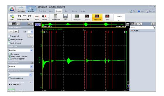
By *zooming in* on the data, one can see the reduced, stored data *before* the trigger, where only the maximum and minimum of the signals is seen and then for a *region with* trigger the *full speed* data can be seen.
