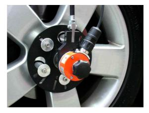
Again, we need to set the *channel setup* for the wheel sensor. This sensor is not defined as standard in DEWESoft, therefore we need to create it with the Counter sensor editor.
