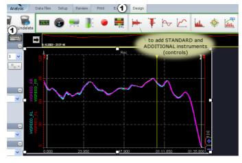
There are all four *wheel speed* measurements. When the recorder is added, the first channel is *automatically* assigned to it. To *deselect* this channel, go to the last icon in channel selector to show channels on current visual control and click on all channels to deselect them.
