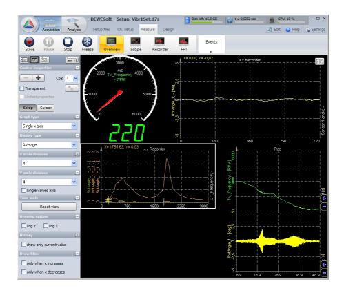
To see it even better, we can add the 3D graph. This graph can only show matrix channels. Order tracking has two of them - OrderFFT and TimeFFT, which can be used as the data sources. Now we can start our run up or run down. Since the color shows the amplitude at a certain frequency and RPMs, we need to carefully choose the *amplitude scale* to show the graph in a nice way. To see also the small amplitude values, the logarithmic y scale is recommended.
