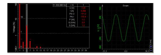
Actually we can calculate the apparent, active and reactive power for *each individual* harmonic. We can also calculate the interharmonics. Those are sine waves or other signals appearing in between the harmonic lines, which are *not covered* by the harmonic calculations.
