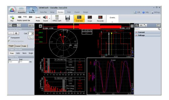
Now let's observe these characteristics at full power. The current is taken from the full cycle and the phase angle between voltage and current is much lower. Also, the current harmonics have dropped significantly are following the voltage harmonics.
