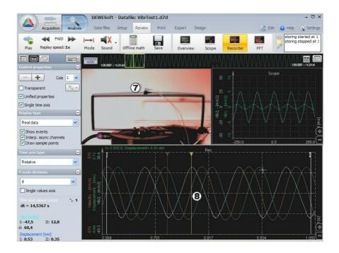
Here, we conducted a simple experiment to get a better feeling about the vibration measurement. In practice, the vibration measurement would surely look different, but we would use the same basic principles as shown in this example.
