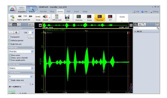
The recorder below shows the RMS of the signal. We can judge from the *average*, *RMS* and *min/max* values what the original signal could be. For example if there is a big maximum and the average value did not grow, we can deduce that there was a short spike in that channel.
