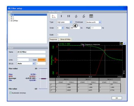
If we show those two filters on the *recorder*, we can see that the signal is nicely *decomposed* to the static load and dynamic ringing. The user can use this technology to *cut off unwanted* parts of the signal or *to extract wanted* frequency components of the certain signal.
