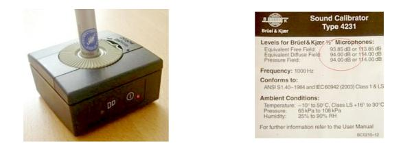
This value is entered *directly* in the Reference value ③ field of the **sound level** module channel setup. Then we *connect* the calibrator to the microphone, and turn it on. We can see the signal directly in the small overview. In our case, it should be a sine wave with a *frequency* of 1000 Hz. Since all the frequency weighted curves are referenced to 1000 Hz, this is a *very usual* frequency for calibrating microphones.
