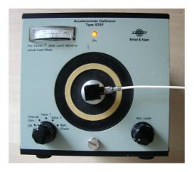
Then we enter in Scaling **by two points** the acceleration level of 7,07 m/s<sup>2</sup> and click calibrate "**from RMS**" (4). The current measured voltage level in mV is written to the second point scaling.
