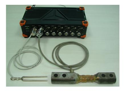
From the amplifier side, we use two 9 pin MULTI modules with isolated input.
