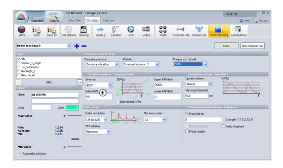
Now let's do some measurements. We have frequency and harmonic channels, therefore we can add the x-y display for displaying the orders. The OT\_Frequency should be used as x reference (first chosen channel of x-y), and the H\_1, H\_2 and H\_3 orders should be used as the y axis. Then we make a run down to observe the orders, where we can clearly see the *peak* at 1800 RPMs that we previously observed in the recorder being the first order of vibrations.
