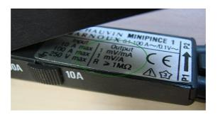
At this range, the sensitivity of the sensor will be 1 mV/mA, which means that 1 mA at *input* will *output* 1 mV at the output. In the **channel setup** we enter that the measurement of current I is in unit A, and leaving the *scaling factor* as **1**. That's all there is to this one. Let's take a look how to scale the shunt resistor.
