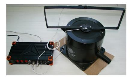
It is always advisable to use a measurement device with *anti aliasing* filter. Otherwise, we can never be sure that the measuring is correct. Quite often acceleration in high frequency range (around 20 kHz) is very high. If a device without anti aliasing filters is used, and samples with lower sampler rates are taken, those high frequencies will be mirrored in the lower range. Especially for the measurements like *modal* analysis this is the most important criteria.
