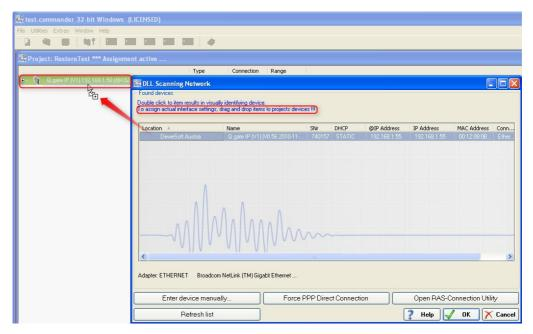
Illustration 350: Drag & Drop the device to assign it to the project
