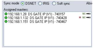
Illustration 109: DSNET: one system without HW-sync cable
