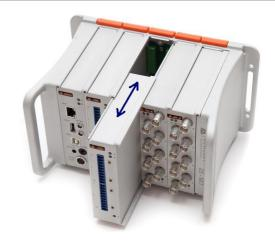
Illustration 301: DS NET: insert/remove module
