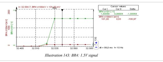
Another important function that is related to these module range min/max values is the Range Error check function which is ON per default for all channels. This function is very useful to detect a broken sensor connection or an out-of-range condition.
