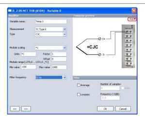
Illustration 138: Alternative connector example (TH8 thermocouple)
