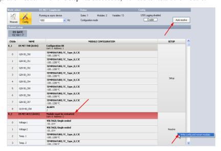
Illustration 154: DS NET plugin: restart module after replacing a module
