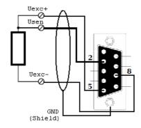
Illustration 226: BR4-D Strain gauge with half bridge completion adapter BR4-D-120/BR4-D-350
