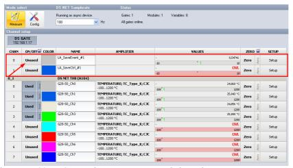
Illustration 305: DS NET plugin: Logger control channels
