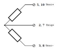
Illustration 224: BR4 Strain gauge with half bridge completion adapter BR4-120/BR4-350
