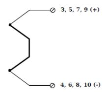
Illustration 245: TH8 differential thermocouple measurement
