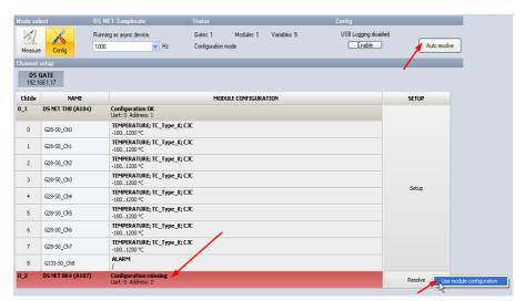
Illustration 151: DS NET plugin: Config Mode after adding a new module
