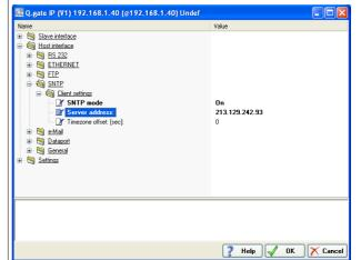
Illustration 84: test.commander: SNTP configuration
