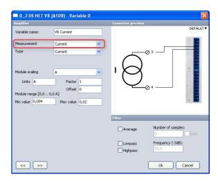
Illustration 232: V8 Channel Setup For Current Measurement
