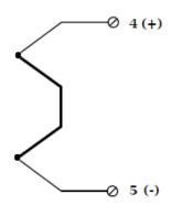
Illustration 183: ACC2 differential thermocouple measurement
