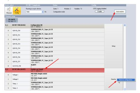
Illustration 155: DS NET plugin: Config Mode after removing a module
