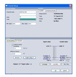
Illustration 130: DS NET plugin: Measure Mode -Channel Setup
