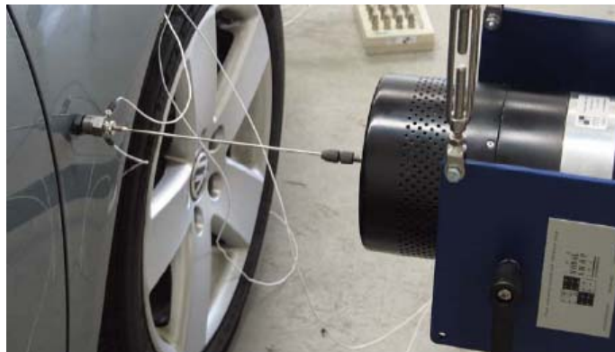
Figure 6 – A typical shaker measurement set up with stinger
