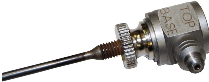
Figure 7. PCB 208 series force transducer, shown installed on a TMS 2155G12 modal stinger
