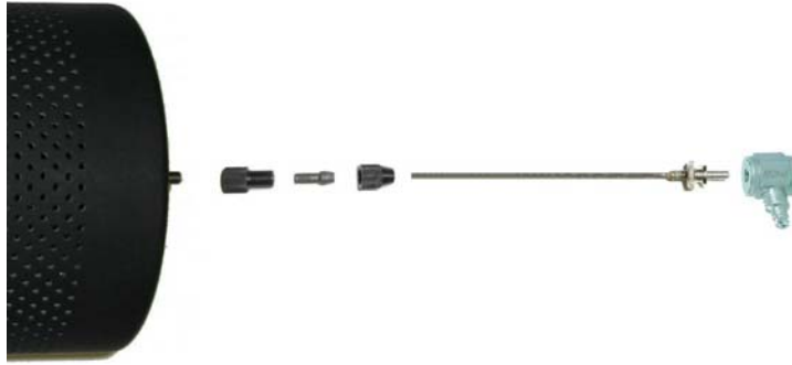
Figure 2. Exploded view of shaker, two-part chuck, collet, stinger and force transducer.
