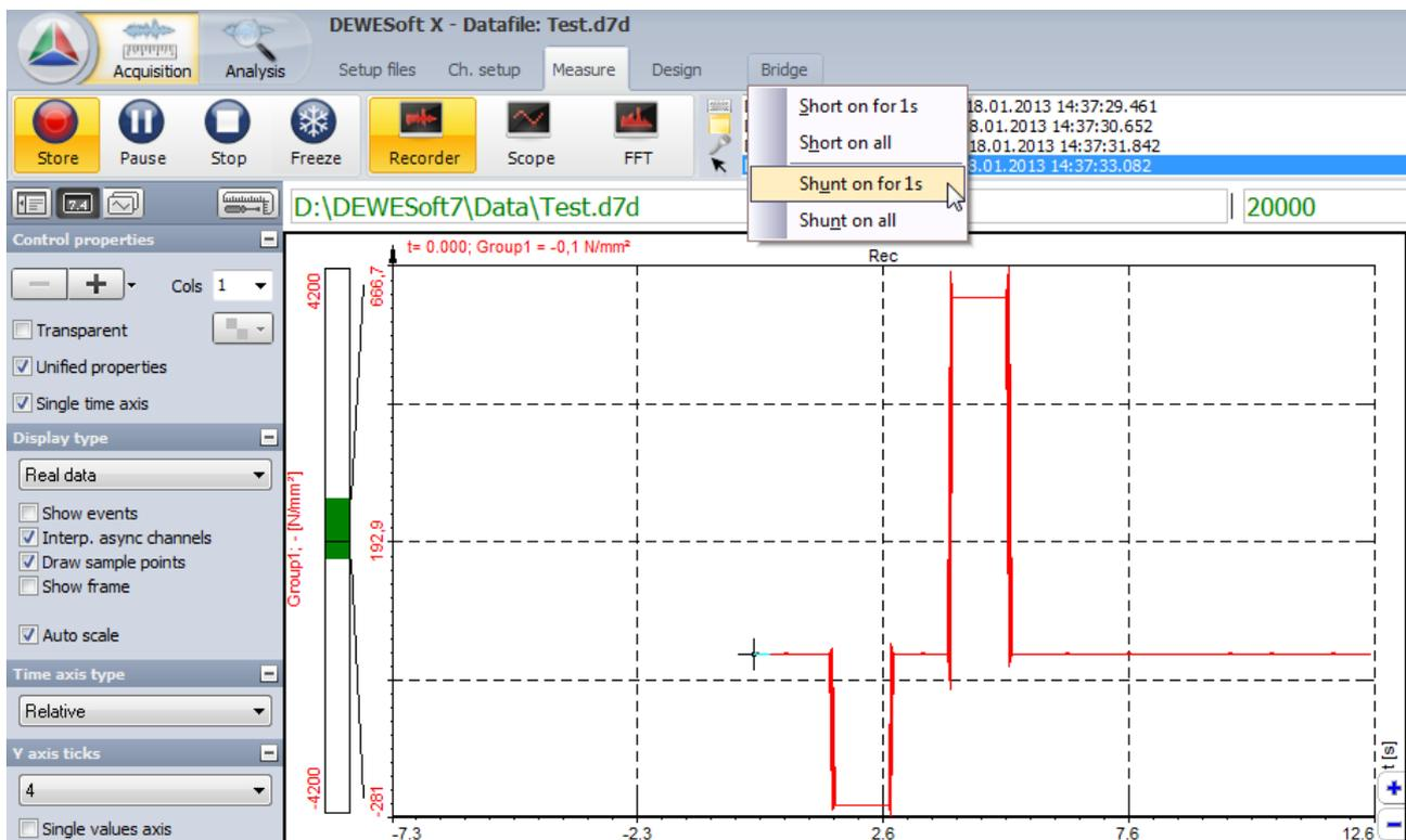
At the end of the measurement – when you are still storing (!) – do again a "Short on for 1s" followed by a "Shunt on for 1s".
