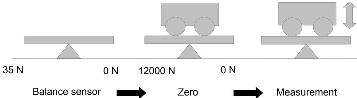
Imagine, we have a force transducer with strain full bridge output. It will measure the weight in our experiment.
