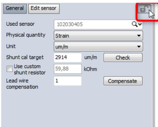
Enter the calculated 2913,9955 um/m in the field "Shunt cal target" and press <Enter>. The resistor is OK with 59,88k.
