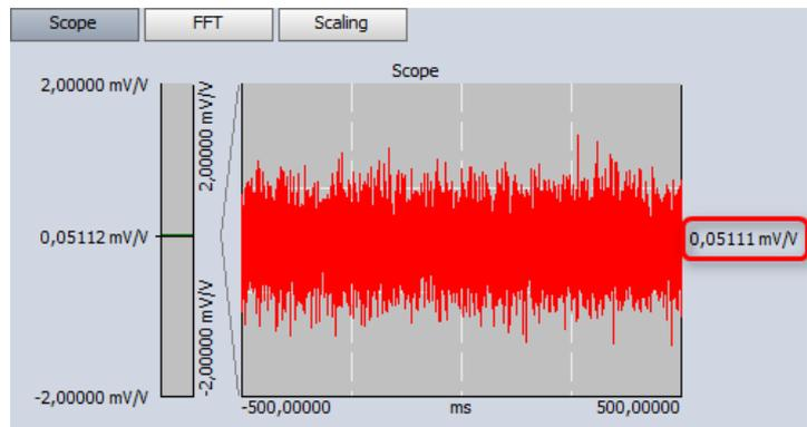
2. Then exit the channel setup and do the "Balance amplifiers", it takes some seconds.
