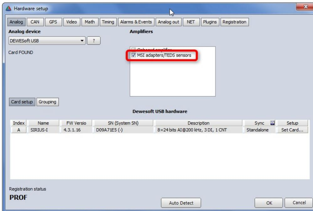
Start DEWESoft; here the sensor with TEDS (a tuning fork with strain gauge applied + TEDS chip inside sensor connector) is plugged into channel 8:
