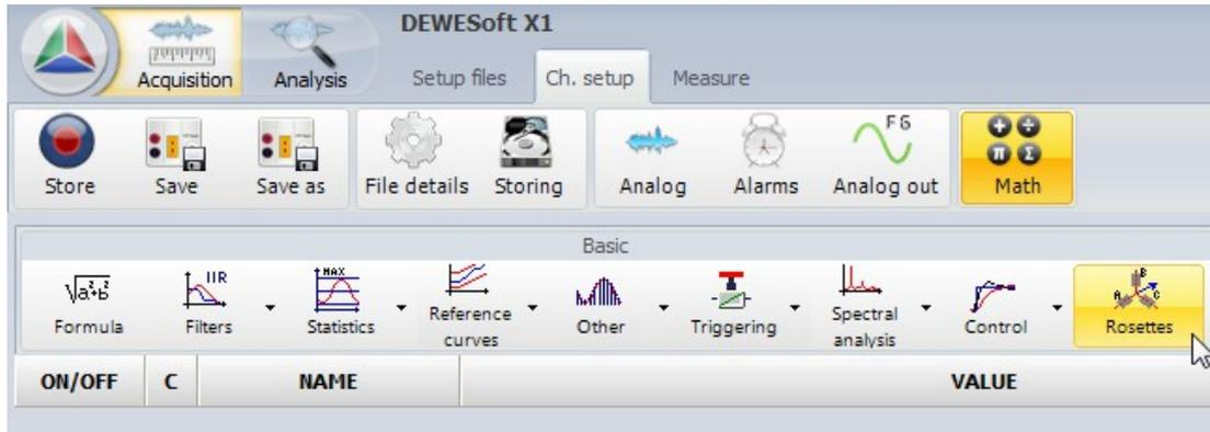
Simply select the 3 strain or stress input channels and the orientation of the elements.
