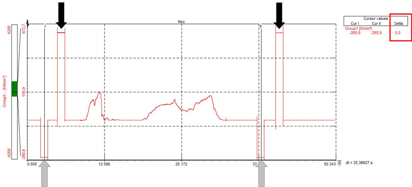
Then move the cursors to the Shunt positions (black arrows), repeat the procedure to also check the Delta of the Shunt measurement.
