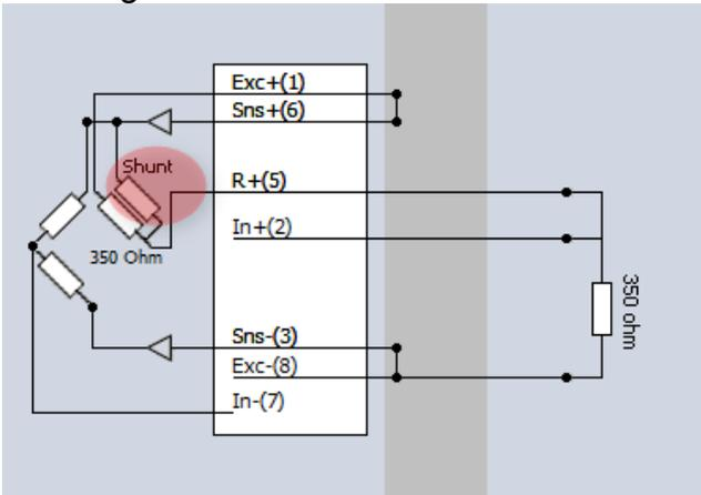
The idea behind is to "shunt" a resistor of known value parallel to one resistor of the bridge to achieve a known, calculateable unbalance.
