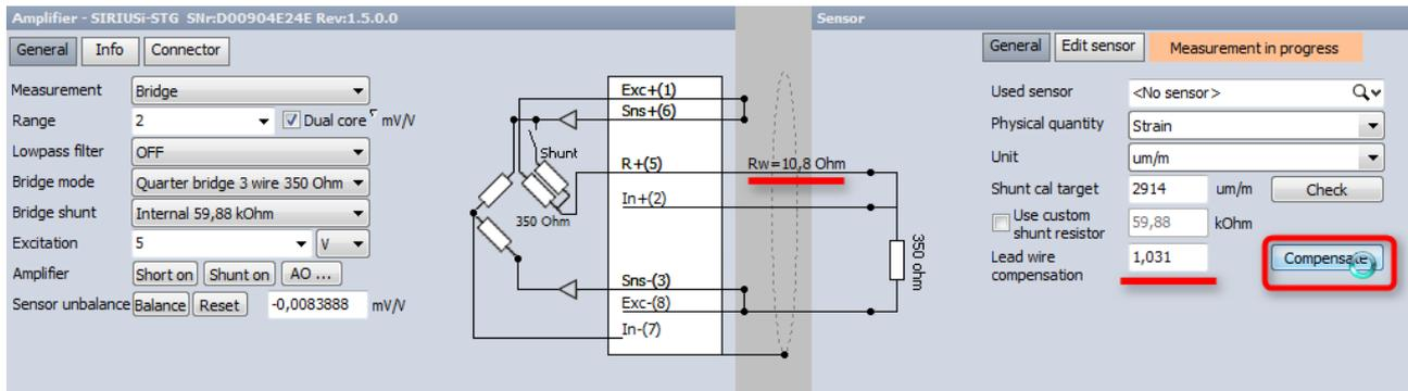
The correction factor is calculated (1,031 in our case) and the measured resistance (10,8 ohms) displayed.
