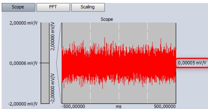
4. If you want to reset the offsets again, please go to Settings -> Hardware Setup -> Analog -> and click the "Set card..." button on the right side. In the tab "Ampl. Balance" you see a list of all the applied offset corrections for each channel.
