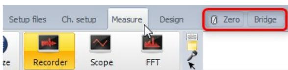
If the "Zero" button is not there, most likely sensors from the sensor database / TEDS sensors are used, and changing the offset is not allowed. Check sensor settings in Channel setup or Sensor editor.
